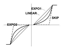
The *optional* **VAR**iable ratio adjusts the steering gain according to the speed command. At slow speeds steering gain and effectiveness is maximum. At full speed the steering gain is reduced. This places the less stable high speed turns beyond operator reach for safety.
