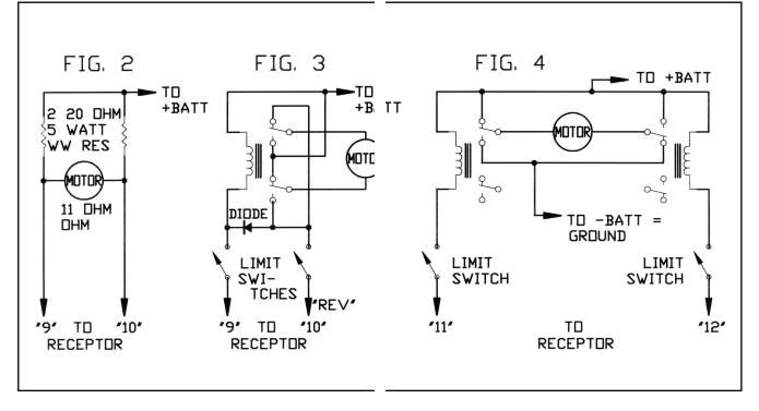
video cameras. The resistors provide automatic current limiting and un-equal resistor values can be used for different forward and reverse speeds. Experimentation is required but for a 12V battery bridge resistors should be greater than 15 ohms; 24V battery - 30 ohms. Put a MOV across the motor brushes.
