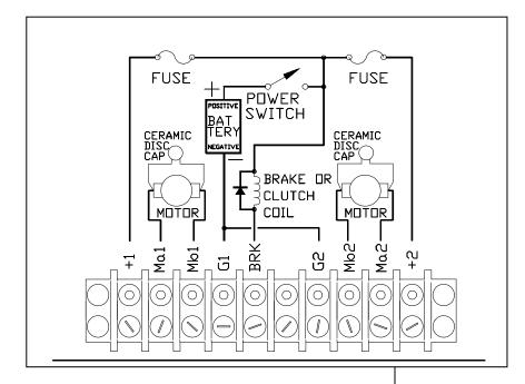
the +1 and +2 power ter minals; start with a 5-10 amp fuse and work your way up to the smallest fuse amperage fu se which will support your norm al operation. NAPA auto parts has a variety of plastic cased hi-a mp fuses. Va ntec doesn't reco mmend thermal Circuit Breakers.
