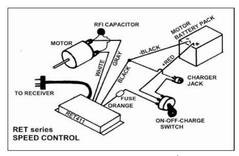
Connect the motor to the controller's white and gray heavy gauge wires. If throttle stick operation is backwards simply reverse these two motor wires; do *NOT* reverse the battery connections.
